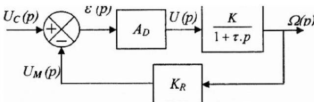
6.g)  $T_{BF}(p) = \frac{\Omega(p)}{U_C(p)} = \frac{\left(\frac{A_D K}{1 + \tau p}\right) \epsilon(p)}{U_C(p)} = \frac{\left(\frac{A_D K}{1 + \tau p}\right) [U_C(p) - U_M(p)]}{U_C(p)}$
